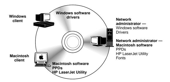
The printer CD-ROM contains the software components and drivers for end users and network administrators. The printer drivers provided on the CD-ROM must be installed to take full advantage of printer features. The other programs are recommended, but are not required for operation. Check the installation notes and Readme files on the printer CD-ROM for more information.
