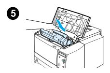
Over time, particles of toner and paper accumulate inside the printer. This can cause print-quality problems during printing. Cleaning the printer eliminates or reduces these problems.
