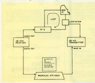
Fig. 1. Station wiring.
