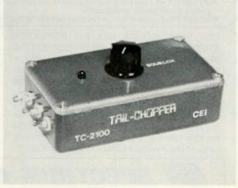
Tail-Chopper squelch-tail eliminator from Circuit Electronics.
