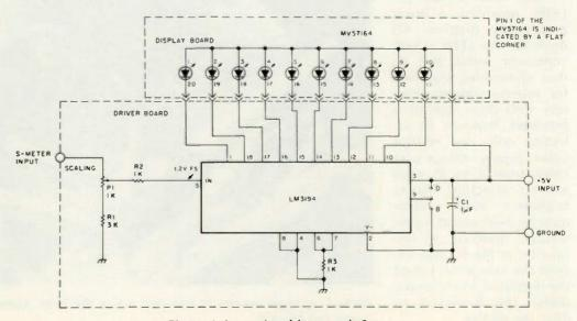
Fig. 1. Schematic of bar-graph S-meter.
