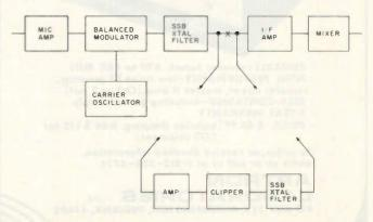
Fig. 4. Rf clipping can be added to most SSB transceivers by breaking the i-f chain after the SSB filter and adding the stages shown.
