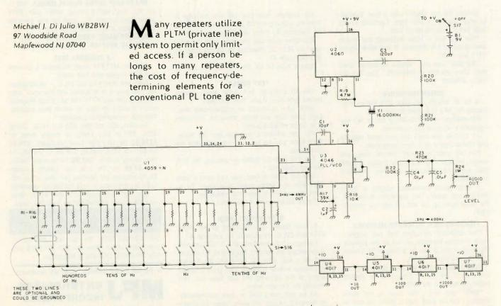
Fig. 1. Synthesized tone generator schematic.
