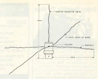
Fig. 1. The Flexi-Plane with BNC connector.
