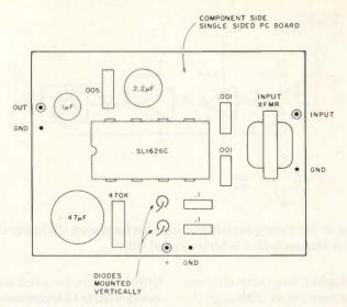
Fig. 3. A typical parts layout for the af compressor. The layout is exaggerated, of course, but any similar layout where the input/output is kept well separated will suffice.
