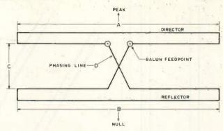
Fig. 2. The ZL Special is composed of two phased driven folded dipoles made from 300-Ohm twinlead. The driven director is 4.4% shorter than a half-wave element and the reflector 1.7% longer. Formulas for dimensions in inches: A  $= 5446 \div MHz; B = 5794 \div MHz; C = 1266 \div MHz; D$ = 1266 ÷ MHz. Dimensions for 146.5 MHz are: A = 37-1/8"; B = 39-1/2"; C = 8-5/8"; D = 8-5/8".
