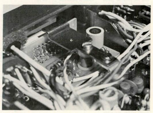
Photo C. Completed circuit installed within the 7400. About 4/10" is needed between the board and bracket.
