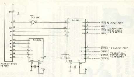
Fig. 1. Schematic of strobe generator circuit. Unmarked capacitors are 0.1-uF, 25-volt disc ceramic
