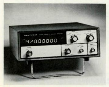
The Heathkit® 512-MHz portable frequency counter.
