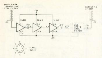
Fig. 5. Extremely simple but high-performance rf-clipper circuit shown with a 9-MHz crystal filter.
