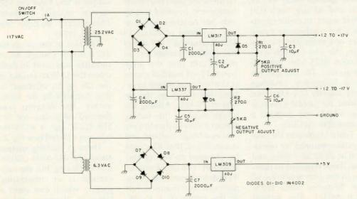
Fig. 1. Tri-voltage power supply schematic.
