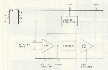
Fig. 1. Internal stages in the Plessey SL1626C af compressor.
