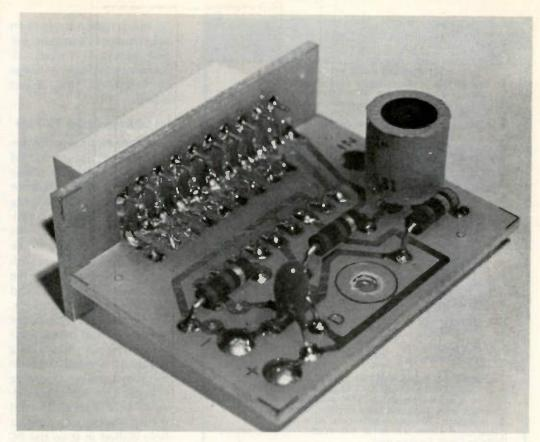
Photo B. The two boards joined using the rows of large pads. The IC is mounted underneath the board.
