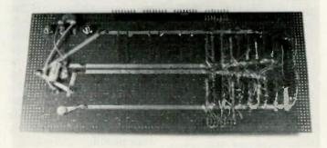
Photo B. Bottom view of the I/O board. The 2 × 20 header is at the right. The electrolytic and ceramic capacitors for the regulator circuit are at the left. Power buses are 1/8"-wide adhesive copper strips made by Circuit-Stik<sup>TM</sup>. Small white spots are paint used to mark correct positions for the sockets and headers. Terminating resistors (input port) were added after the photograph was taken.
