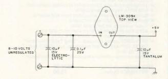
Fig. 3. Schematic of power-supply regulator. The 10-uf capacitors are tantalum and electrolytic; the 0.1-uF capacitor is disc ceramic.
