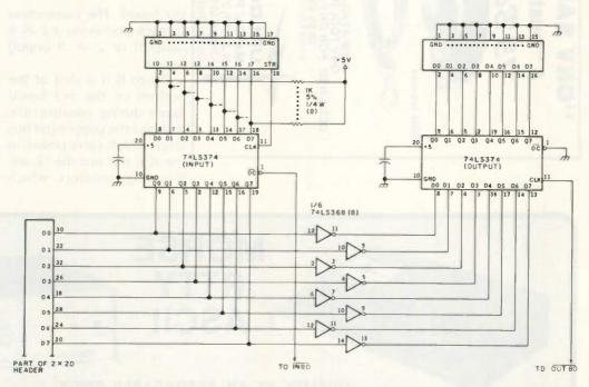
Fig. 2. Schematic of port function circuit. Unmarked capacitors are 0.1-uF, 25-volt disc ceramic. Tie enable inputs (pins 1 and 15), unused data inputs (pins 2, 4, and 6), and ground pin (8) of the 74LS368s to ground. Tie +5-volt pin (16) of each 74LS368 to +5 volts and bypass to ground via a 0.1-uF, 25-volt disc ceramic capacitor.
