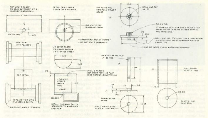
Fig. 3. Construction details for cavity wavemeter.
