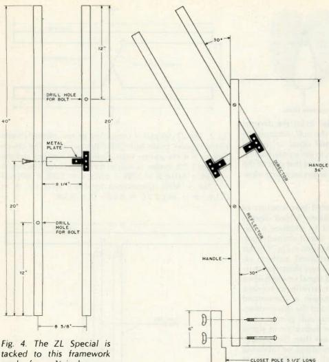
Fig. 4. The ZL Special is tacked to this framework made from 34-inch-square wood. Dimensions given are for an antenna cut for 146.5 MHz.
